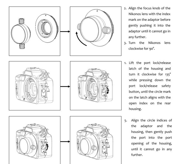
4. Turn the port lock/release latch anticlockwise for 135° to the "lock" position.
